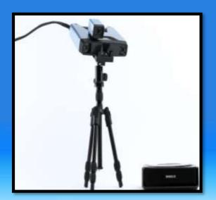
A handheld 3D scanner is a portable device that uses laser or structured light technology to capture three-dimensional data of objects. The 3d scanner allows users to create high-resolution, accurate digital models of physical objects for various applications such as 3D printing, reverse engineering, and product design.
